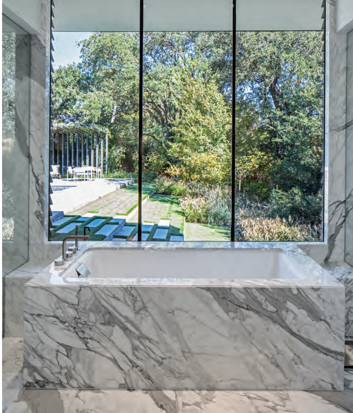
The master bathroom's Kohler tub with Fantini hardware, all from TKO Associates, is encased in marble that flows to the floor and walls. The architect had the glass for the windows, which provide views of the pool and pergola outside, glazed in place for a frameless look.
